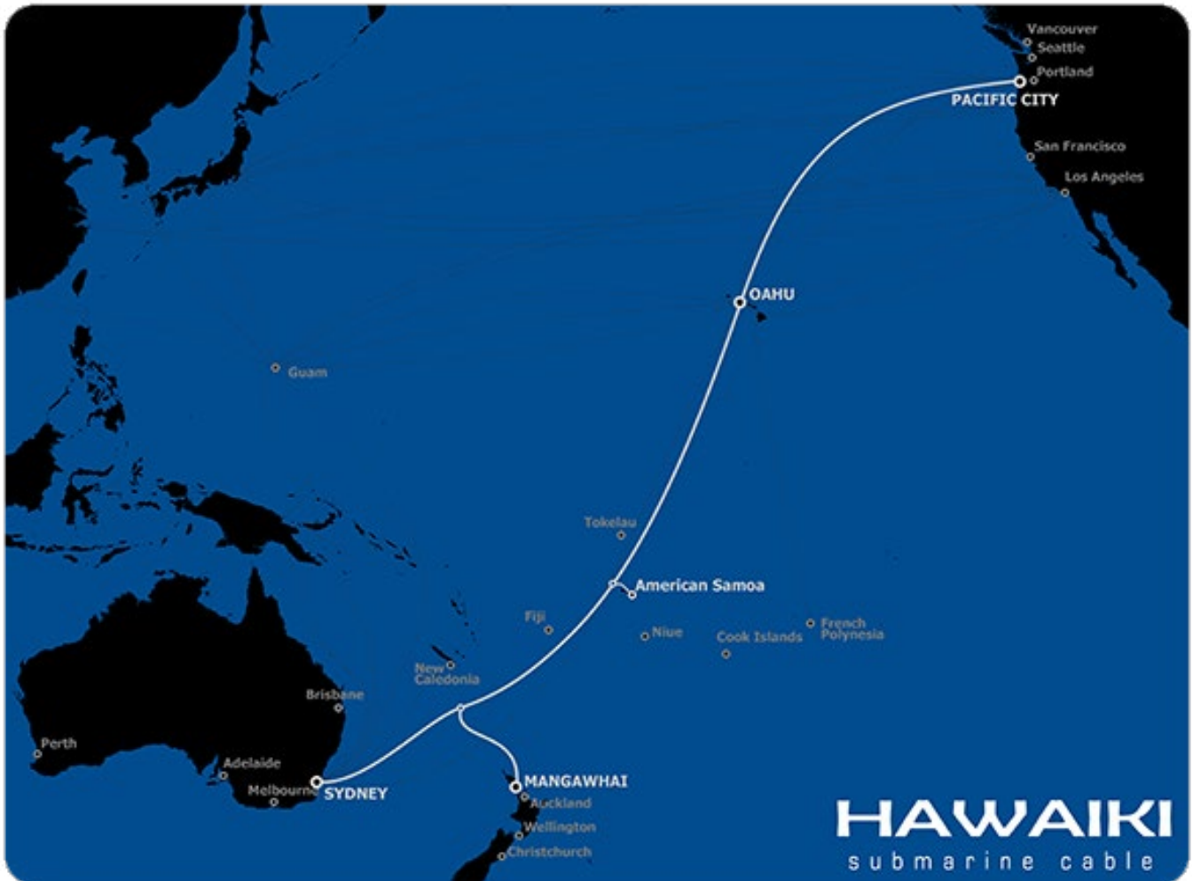
Figure 1. Hawaiki Submarine Cable connecting Australia and New Zealand to US through American Samoa and Hawaii.
